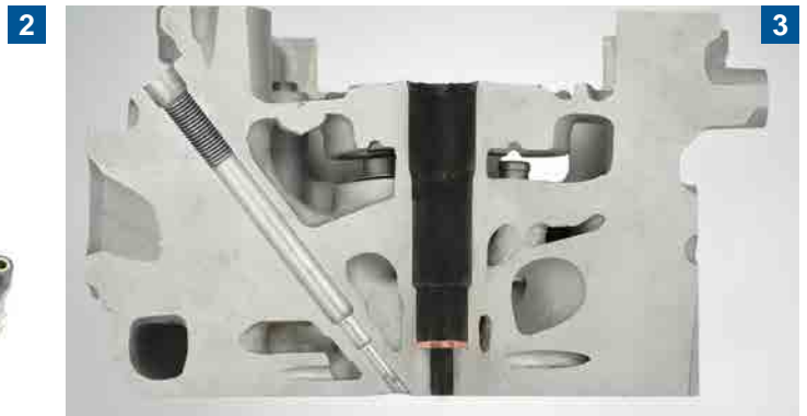
Cylinder head cross section with soiled injector shaft
